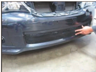
Picture #7: Place the lower grille into the bumper opening as shown
