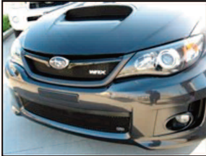
Picture #19: 2011-2012 Subaru WRX shown here with hood scoop, lower and upper black mesh grilles.
