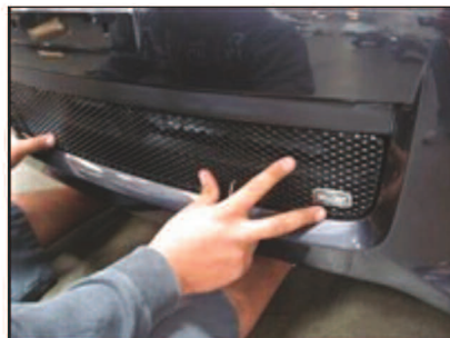
Picture #8: Hold lower grille securely in place.
